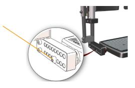
This picture shows the bracket reaching backwards, allowing for longer right leg where the right leg support and its calf pad go forwards: – suiting a user with longer right leg.
