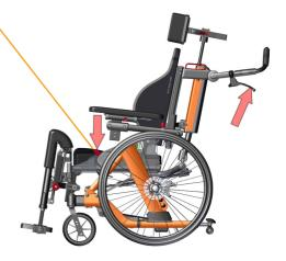
Always use the parking brake when the wheelchair is left without attendant standing close. Lock the parking brakes on both sides.
