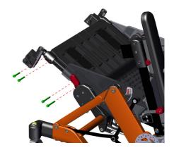
Adjusting leg support extension pieces allow for adjusting for knee joints not being aligned with the leg support knee joint.
