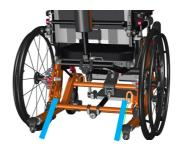
In the rear: Hook on a hook / carbine hook into the car fixing loops on the frame. The angle of the straps should be close to 45°.
