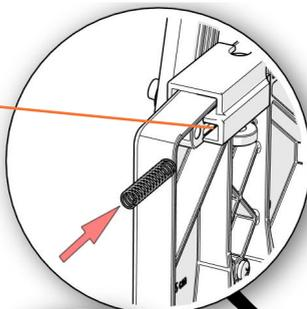
Press the plastic bolt into the hole on the footplate where the spring ends. A firm blow with a hammer fixes it permanently.
