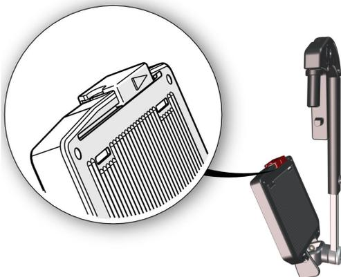
Insert the spring into the tunnel under the lockunit on the underside of the foot plate.
