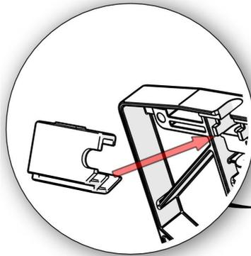
Position the red lock unit under the foot-plate to have the pointing edge hooked behind only one of the noses on the foot-plate.
