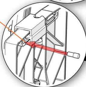
Pull the lock a couple of times to control that it snaps back into lock position.
