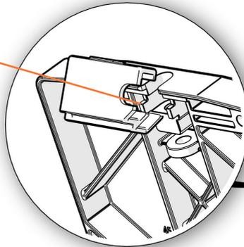
Push the red lock firm against the footplate to have it snap over the edge ( see the red arrow) and into the groove on the top of the footplate.
