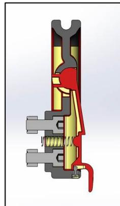
Raise the lever so far that you can insert the spring into the centre hole of the armrest bracket. Then, move the lever down again, making sure that the little buckle at the backside of the lever will meet the spring right in the middle. This will keep the spring in position.
