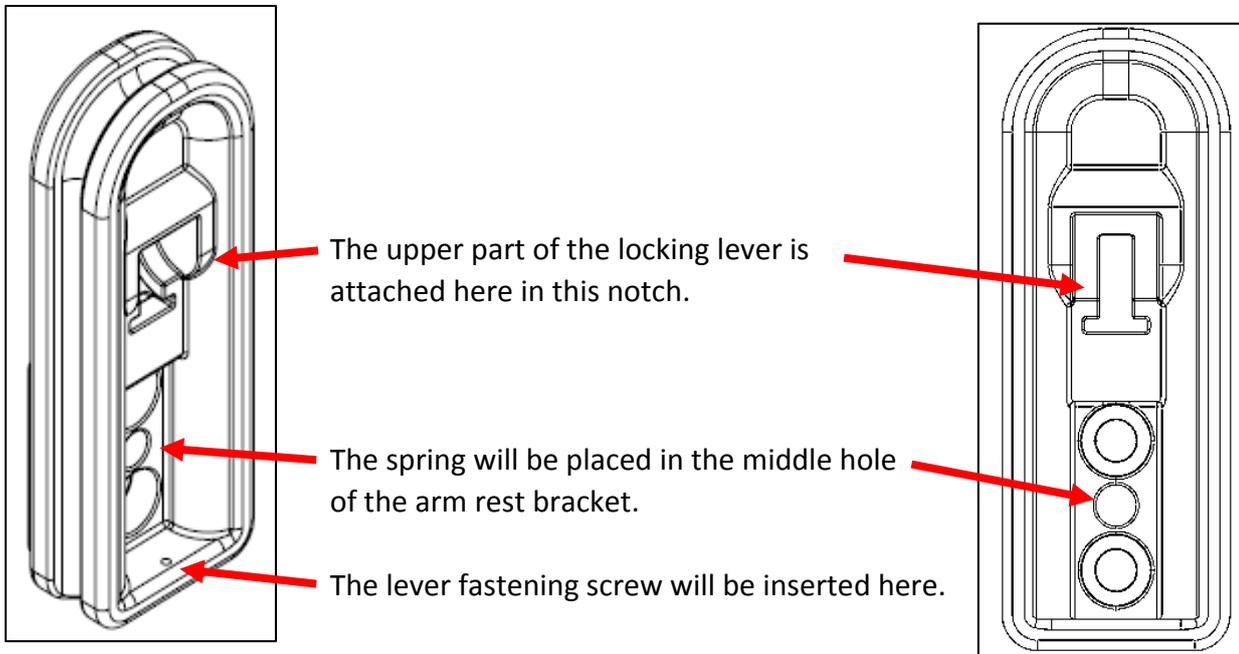
In the following 2 pictures you can see where the locking lever is inserted into the armrest bracket and where the spring as well as the lever fastening screw is placed.
