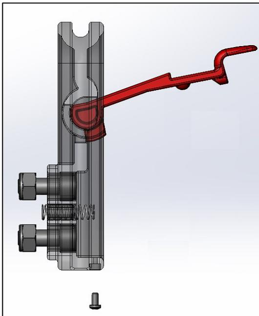
Start the mounting by placing the locking lever horizontally against the armrest bracket and slide it into the recess provided in the bracket for this purpose. Then fold the lever down.
