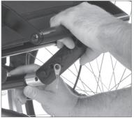
Lock the backrest by pushing the locking bolt through the plastic bracket and gas spring locking head.
