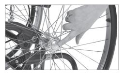
To check that the main wheel is properly attached to the hub, remove the finger from the central knob and pull at the main wheel.
