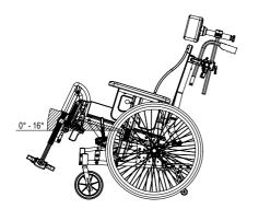
A backward tilted seat unit gives a steeper seating angle in relation to the surface, and prevent sliding of the wheelchair user.
