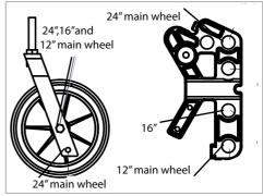
If it is required to change position of the main wheels or to change to a different size of main wheels, unfix the hub bushing including washer and nut. Remove the hub bushing and mount it in the required position.
