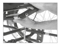
Lock the backrest by pushing the locking bolt through the plastic bracket and gas spring locking head
