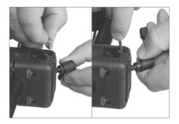
The head support bracket is fixed by tightening the four screws two by two diagonally so the bracket is fixed with the same strength divided on the four screws.
