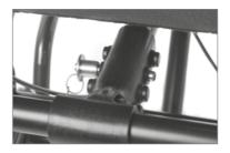
The back rest hinge has 4 holes. The hole positions are in accordance with the holes in the plastic bracket. If the locking head of the gas spring is mounted in the inner hole of the plastic bracket, the back rest hinge should also be mounted in the inner hole etc.
